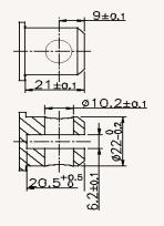
2=clevis head, width 6.2, depth 20, hole dia 8.2MM
