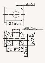
2=clevis head, width 6.2, depth 18.0, hole dia 10.2MM
