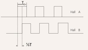
Brown: motor+ Blue: motor-Red: VCC 5V+ Green: GND 5V-White: hall signal output A Yellow:hall signal output B
