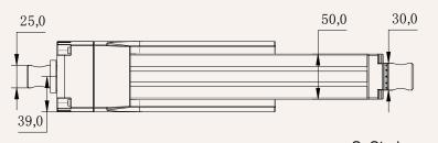
S: Stroke L: Retracted length L=Stroke +250mm
