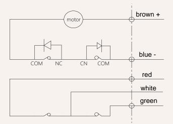
1.brown: motor + 2.blue: motor -3.when extend: brown+, blue-4.when retract: blue+, brown-5.white:common line 6.white and red: extend to the end signal 7.white and green:retract to the end signal
