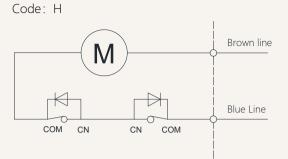
Schematic diagram of the internal circuit of the Hall signal
